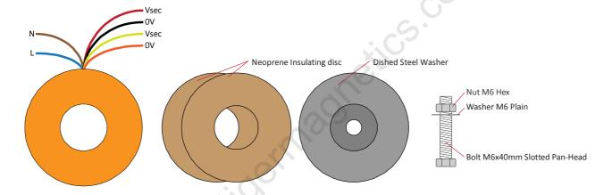
Primary Winding Input Voltage Range: 207V–253V (230V ±10%) @ 50/60Hz
